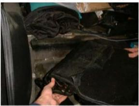
4. Remove the rear centre console: Open the console lid and lift the tray covering. Remove the 4 screws that fix the console to the tunnel (picture 4A). Carefully lift the console, while guiding the seat belt receivers through the console apertures (picture 4B). Mark the position of the cigarette lighter wires and pull them off (picture 4C). as you pull away the console make sure you note the position and recover the plastic washers (picture 4D).
