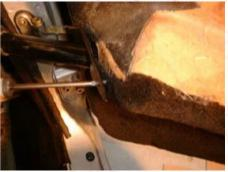
3. Remove the rear seats: Flip the seatbacks forward in their flat position. Remove the Allen screw on the outside (picture 3A). Tilt the seat and move away from the centre pin to remove (picture 3B). The seat bottoms can simply be pulled out.
