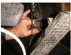
6. You can now remove your old carpets. Removal of your old carpets is easiest by reversing the installation sequence below. As you remove your old carpets take care not to pull off sound deadening material. If you have difficulty pulling the material off it may help to use a knife to cut trough the hardened glue. Do not throw away your old carpets. 'reading' your old carpets may help to install you new ones to perfection.
